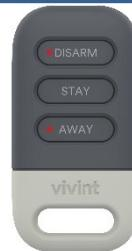
The SKEY2 also provides added protection by letting you send an encrypted panic signal to the panel when the first and third buttons are held down.
